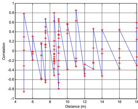
Figure 10. Shadowing Correlation Coefficient as Distance Function
