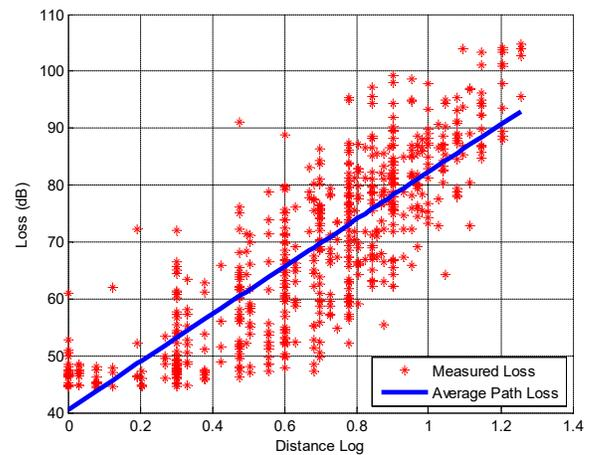
Figure 6. Path Loss as Distance Function
