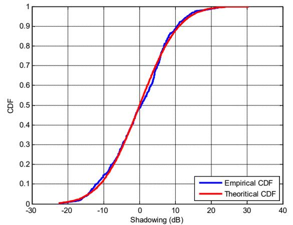
Figure 9. Shadowing CDF Empirical vs. Theoretical degree of 0,05 is 0.053. It can be seen that  $D_2 < c_{n,\alpha}$ . So Thus verified that the obtained shadowing model has a normal distribution in logarithmic scale. This CDF graph can be seen in Figure 9.
