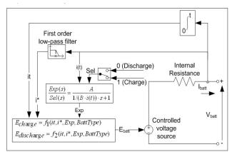
Figure 7. Schematic model of battery on MATLAB
