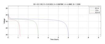
Figure 8 characteristics of the battery discharge with different discharge currents
