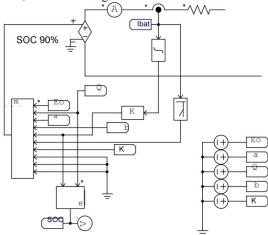
Figure 9. Modeling battery on PSIM
