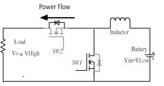
Figure 5 Boost mode from bidirectional converter
