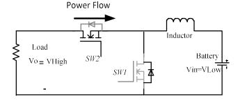
Figure 6. Buck mode from bidirectional converter
