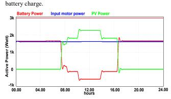
Figure 16. Curve shows the relation between PV power, Battery power and motor absorbed power within 24 hours.
