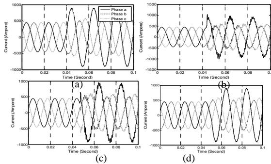
Figure 3. Current shape differences based on Fault Inception Angle
