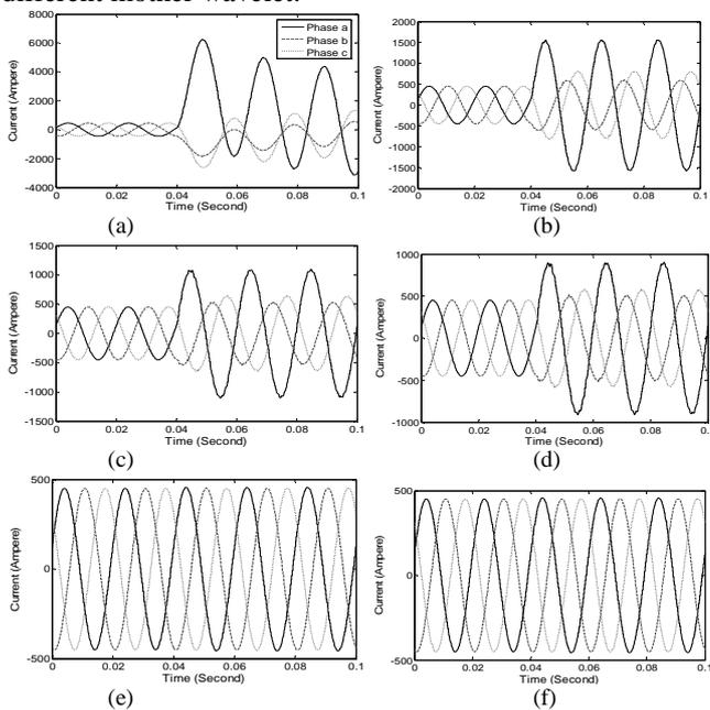
Figure 4. Current Value differences based on fault resistance ( $R_f$ )
