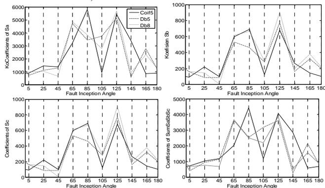
Figure 7. The influence of Fault inception Angle to absolute value of coefficient S
